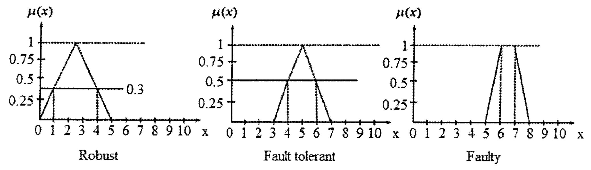
Reliability is measured as  $r = R \cup FT \cup F$ . Determine the crisp value of r using centroid method, COS method and weighted average methods of defuzzification. (5 marks)
